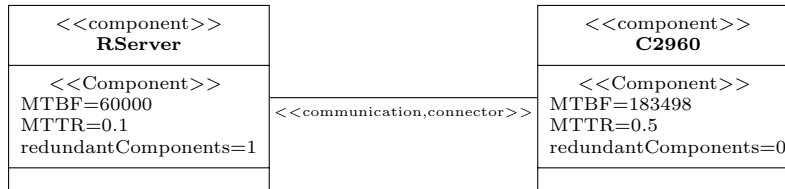
Fig. 7. Predefined network elements represented in UML Class Diagram
