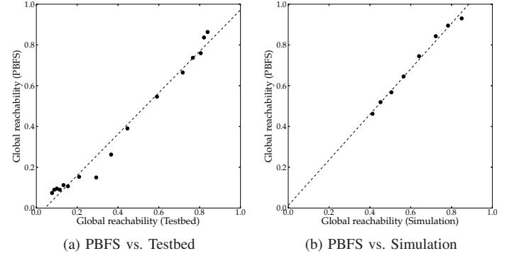
Fig. 4: Comparison of global reachability predicted by PBFS (y-axis) and achieved in reality, simulations (x-axis). A point constitutes the reachability for a single scenario.
