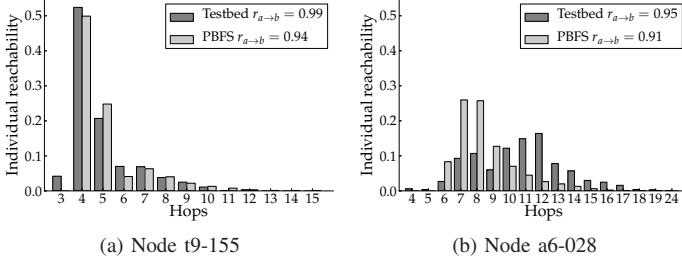
Fig. 6: Exemplary path length distributions for NWBs to nodes t9-155 and a6-028.
