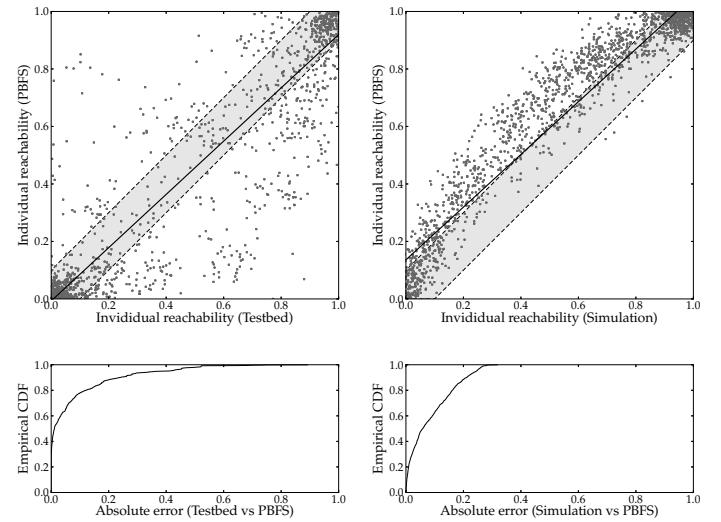
Fig. 5: Comparison of individual node reachabilities predicted by PBFS (y-axis) and achieved in reality or simulations (x-axis) across different scenarios (top). Corresponding CDF plots for the absolute differences shown in the bottom graphs.
